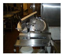
Restaurants use many types of equipment that have machine guarding. Food processors, choppers, slicers, grinders, mixers, compactors have moving parts that must be guarded because of their hazardous motions.
